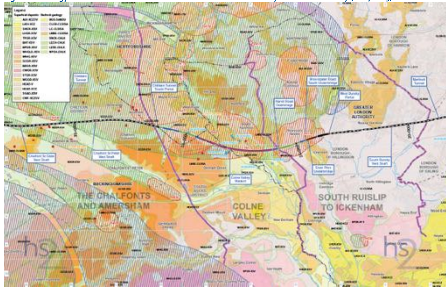
Figure 2: Geology and Groundwater Source Protection Zones in the vicinity of the Colne Valley (HS2, 2013)
